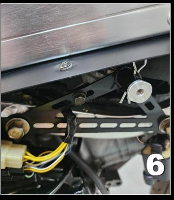
7) And finally fit the M4 bolt and plastic washer to the rear. Adjust the stay as necessary.
