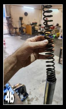
**5)** Remove the fork from the vice and drain all the fluid into a suitable container. You'll need to pump the fork tube and damper rod a few times to help get the fluid out, but there will always be a little fluid left which we can drain once the cartridge is removed.
