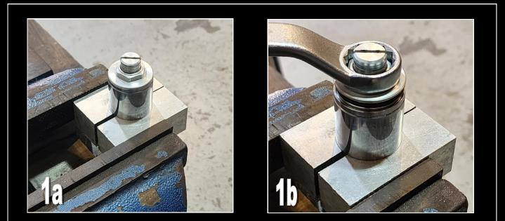
2) Now clamp the forks in the vice vertically and undo the caps completely from the fork tube.
