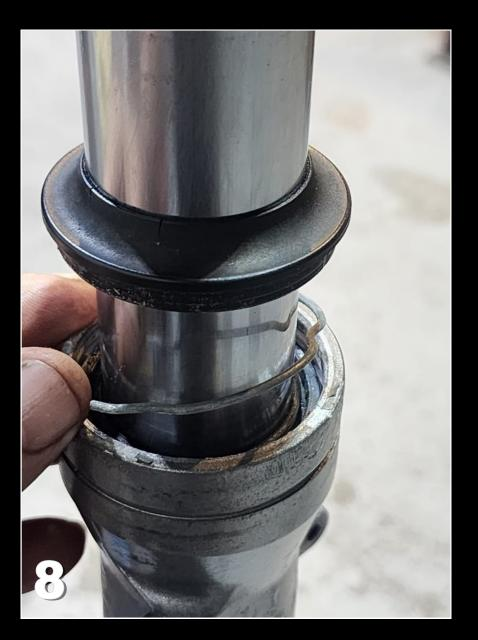
And now we must get a bit aggressive to remove the seal, back up ring and fork bushing. Lock the fork lower in the vice with soft jaws, and use the inner tube as a slide hammer, pulling it abruptly to full extension. This will remove the seal, back up ring and bushing. **9)** Now we have the forks completely apart, so it's good time to clean everything up and check for excessive wear or damaged components.
