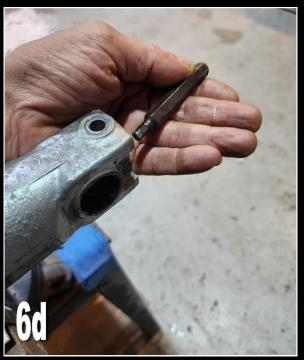
If you get it loose but the cartridge is now turning inside the fork and you can't remove the bolt then try pulling up the damper rod at the top of the fork and keep pulling while turning the M8 bolt. This usually works.
