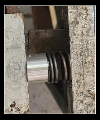
12) Now fit this assembly onto the cartridge. Make sure that it is fully seated and tighten the grub screw. We advise using some Loctite 263 high strength threadlocker compound on the grub screw so that it cannot come loose.
