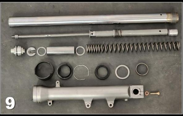
If fully disassembled you should have the following:
