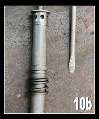
11) Now we can fit the top out spring to the fork shortening piece. This is easily achieved by squashing the two parts together in the vice as shown. Make sure that the top out spring is completely seated and not at an angle.
