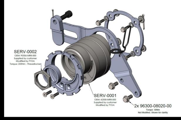
One of the fundamental visual differences between the RC36-2 and the RC30 is the rear wheel. The R36-2 uses a four hole bolt pattern, while the RC30 uses a single nut to hold it in place.
