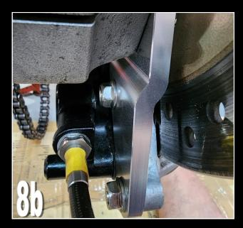
9) Fit the BPSY-0381 Hose Guide to the rear hub pinch bolt and thread the hose through.
