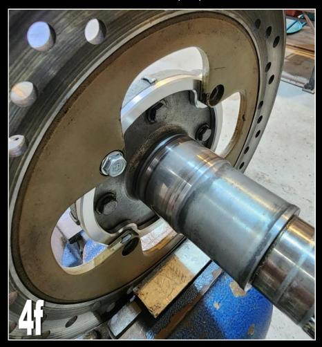
Add a drop of threadlocker to each M6 bolt and screw into the threaded insert. Don't forget to remove the first bolt fitted, apply threadlocker and refit. Torque to 12Nm.
