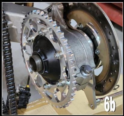
**7)** Now fit the thin shim, locking washer and finally the nut. The nut shown is a standard NC30 nut that has been machined to the same dimensions as the RC30 nut. It does not have the lock wire holes, so it is imperative that this nut is tightened to the correct torque and that threadlocker is used. Torque to 235Nm.
