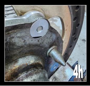
**5)** Apply grease to the needle bearing in the eccentric, and also a light smear of grease on the axle, and fit the assembled axle into the eccentric.
