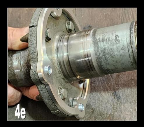
Locate the axle assembly onto the disc and screw in at least one of the M6 bolts to loosely secure the assembly in position.
