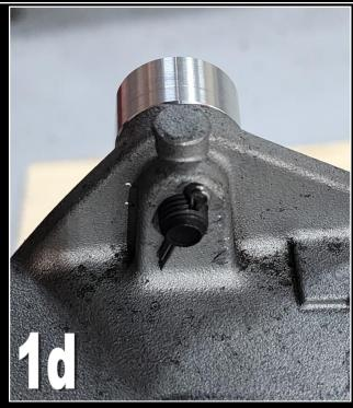
**2)** Now prepare the modified NC30 eccentric. Fit the spacer TYLY-0326E on the left side. The seal will hold it in position. Now slide it into the swingarm from the left side. Note that the bearings should be on the top side, so fit with the bearings at around the 12 o'clock position. It is a good idea to tighten the pinch bolt just a little at this point to stop the eccentric from moving around.
