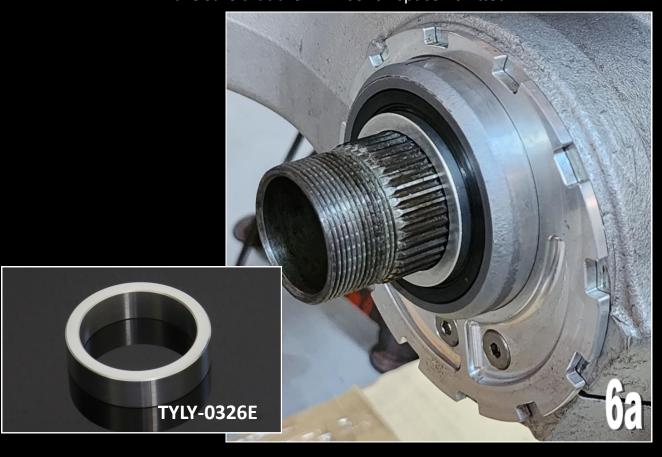
The sprocket should be already mounted to the carrier. Torque the M8 bolts to 33Nm.
